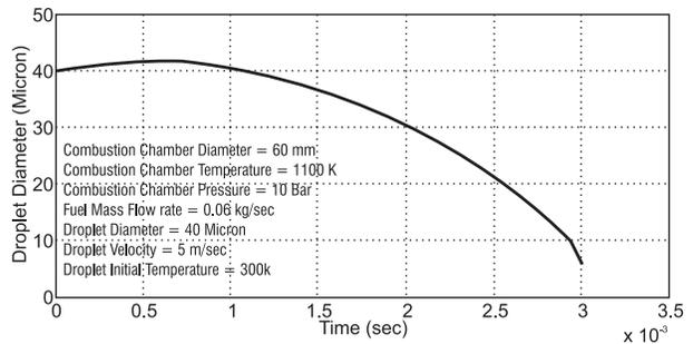
**Figure 3: Fuel droplet diameter in heating phase.**
