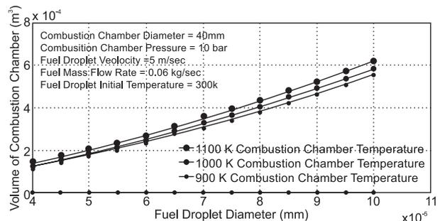
Figure 14: effects of fuel droplet diameter and chamber temperature on volume of combustion chamber.
