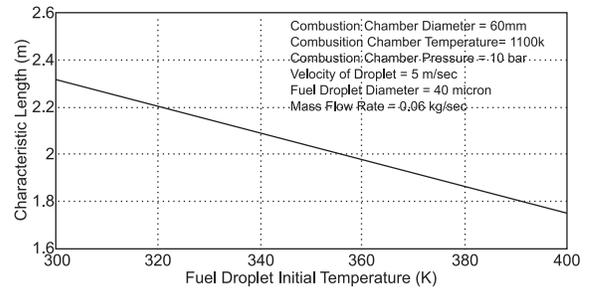
Figure 13: characteristic length with fuel droplet initial temperature.
