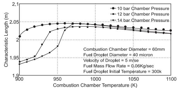
**Figure 11: Unusual behavior of characteristic length against chamber pressure and temperature.**
