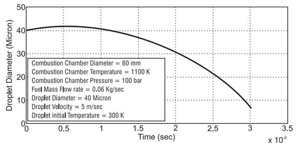
**Figure 5: Fuel droplet diameter with time.**
