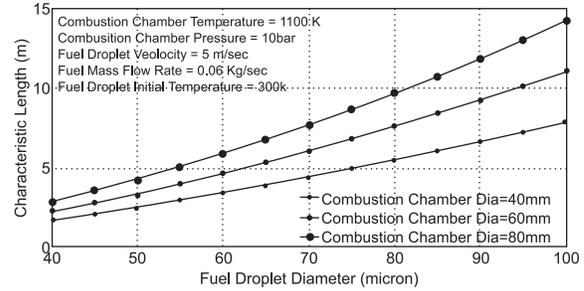
**Figure 9: characteristic length with variation in combustion chamber diameter.**
