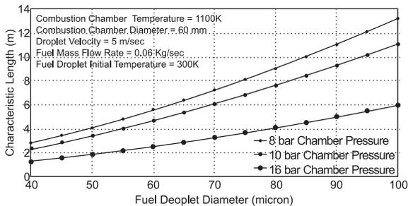
**Figure 8: chamber pressure effects on characteristic length.**
