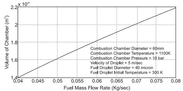
**Figure 10: Mass flow rate effects on volume of chamber.**
