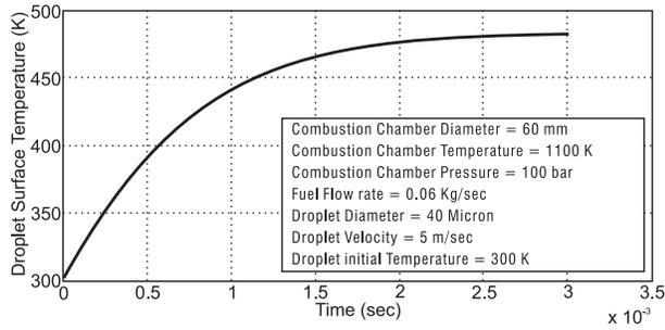
**Figure 4: Fuel droplet surface temperature in heating phase.**
