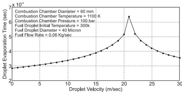
**Figure 7: Effects of droplet velocity on required evaporation time.**
