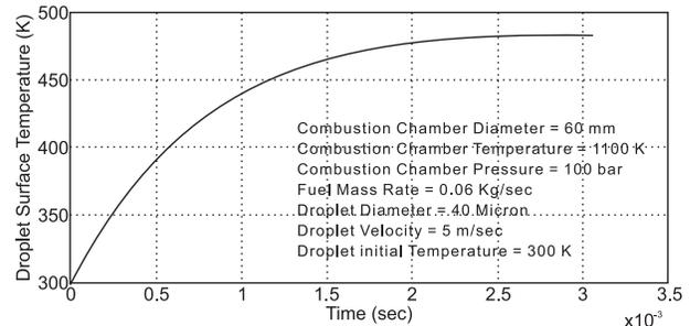
**Figure 6: Fuel droplet surface temperature for its complete life time.**
